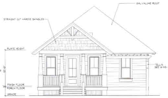
2 FRONT ELEVATION A2-1 SCALE 1/4" = 1'-0"
